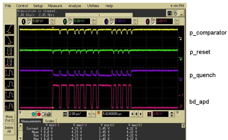
Figure 3: measurement of multiple time firing APD seen at pixel output
